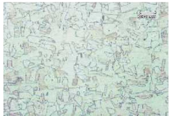
Gambar 4. Struktur mikro sample pipa, 100% fasa austenit
